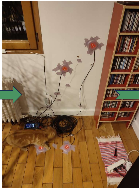
Installed Heat-Flux Meters and remote measurements toolkit
